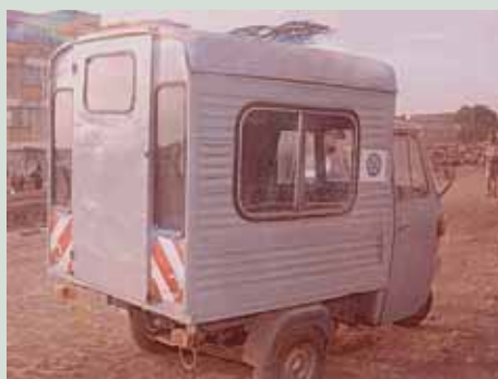
Figure 3.51 Side and rear view of a 3-wheeled motorcycle turned into a prototype accessible van (Courtesy of Wycliffe Kepha)
