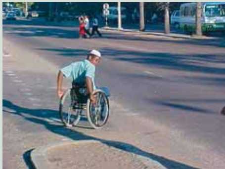
Figure 1.1 High kerbs at pavements force some users to cross the street at dangerous places
