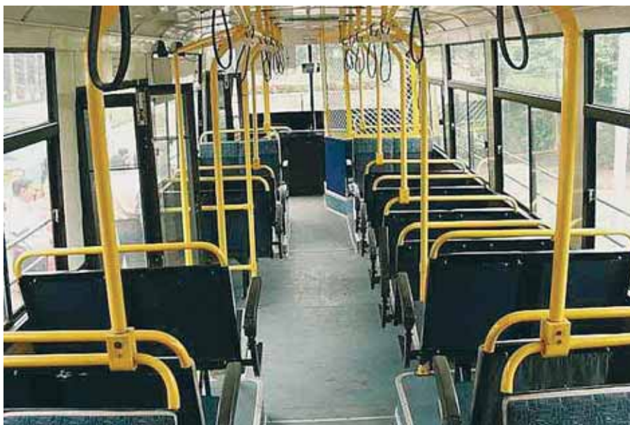
Figure 3.37 Handholds/grips, stanchions and colour contrasted interior, India
